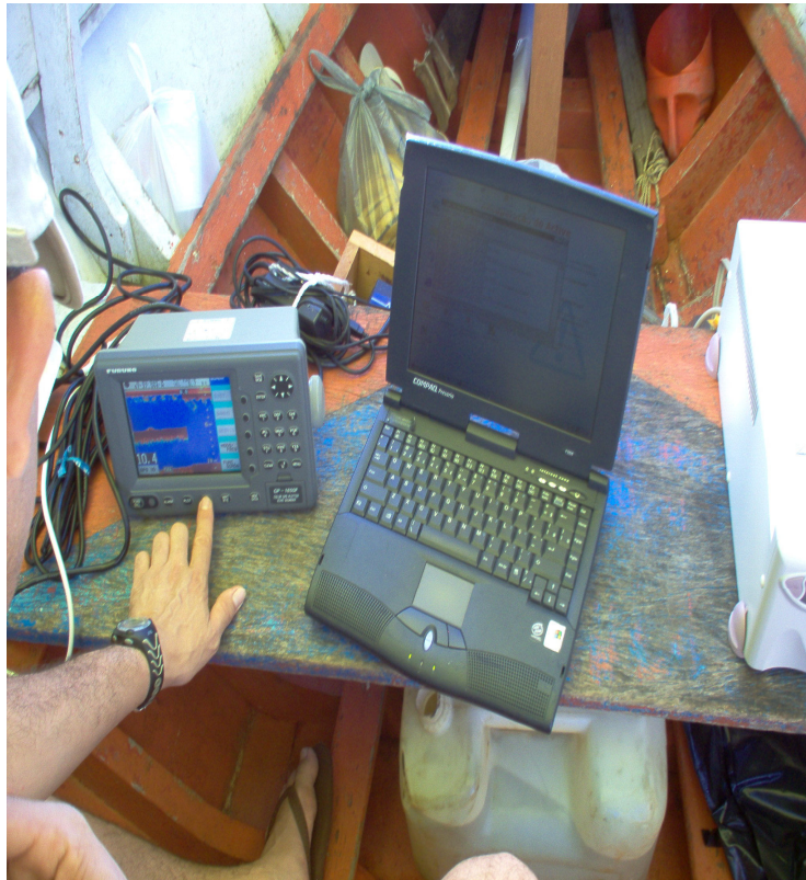
Figura 30: A Ecossonda DGPS/PLOTTER/SONAR, com visor colorido FURUNO GP-1850 F e o nottbook.
