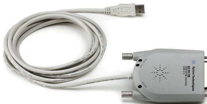
**Figura 3.10:** Interface 82357B USB/GPIB.
