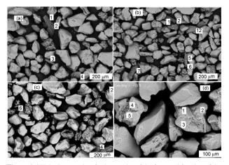
Figure 6. SEM micrographs of sub-samples of the fine sand fraction of the A1, A2 and A3 horizons: (a) and (b): (A1)15; (c): (A2)16 and (d): (A3)17 horizons (backscattering images).
