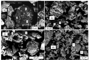
Figure 4. Micrographs showing PyC in the clay fraction from the A2 horizon: (a) circular particle and diatom/D; (b) and (c) tubular porous channels ((A2)/2 sample); and (d) particles having prismatic shapes ((A3)/3 sample).
