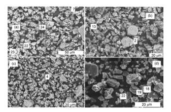
Figure 5. SEM micrographs showing different morphologies of the PyC in the silt fraction (secondary electron images): circular particles (a) and (b): A1/29 sample and other particles from (A2)30 and (A3)31 horizons (c) and (d): (A2)30/ (A3)31 samples.
