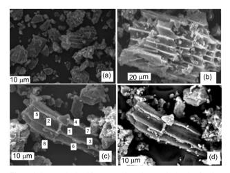
**Figure 3.** Images obtained from secondary electrons in the clay fraction from the A1 horizon in (a) and (c); from backscattered electrons in (b) and (d) showing the PyC particle residue from a burned plant.
