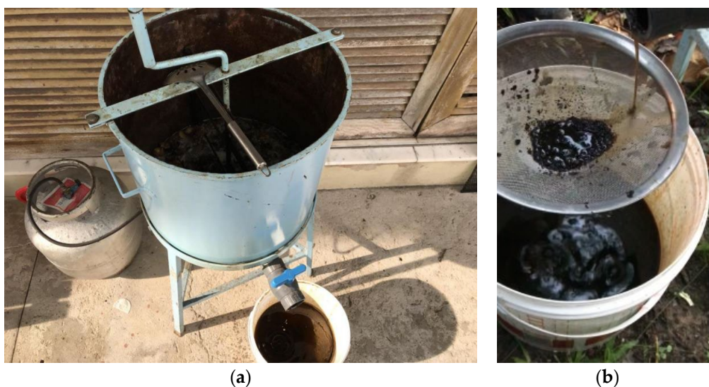
Figure 2. LPG-stirred bed reactor (a) and fat separation by filtering (b).
