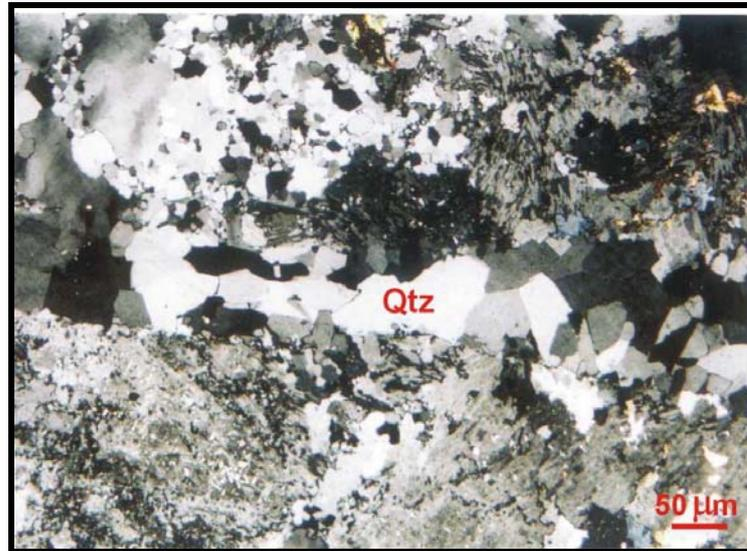
**Figura 46:** Fotomicrografia de veio de quartzo hidrotermal (Qtz) cortando as MVA (Amostra FD-266/366m – Luz transmitida, Nicóis X, 20x).
