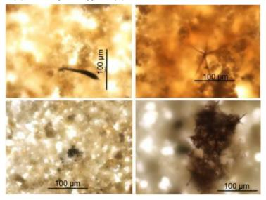
Figure 8 - Painted surfaces after 5, 10 and 15 days of accelerated test with Penicillium sp.
