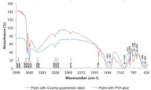
Figure 3 - FTIR spectra of the paints with Couma guianensis' latex and with PVA glue
